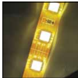
Amber LED lights warn of door movement
